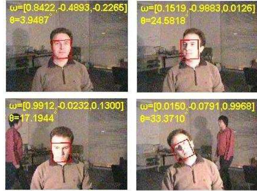
Figure 6. An example of face tracking using GAMs under changes of pose and lighting. The estimated pose is shown on the top of the frames. (Should be viewed on a monitor)
