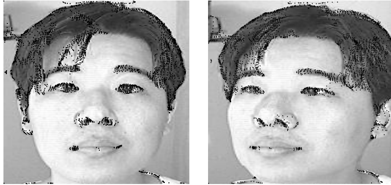
Figure 6.1: The output of the corner finder algorithm on two images obtained from projections of the partial models, represented by small dots.
