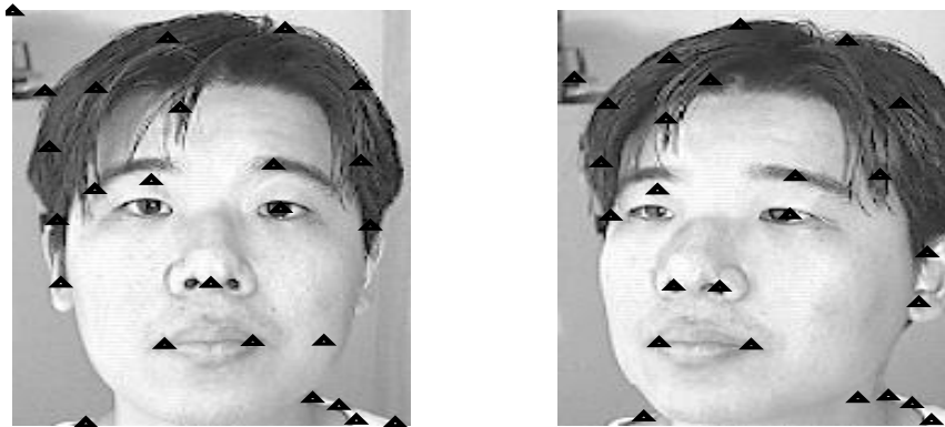
Figure 6.2: Features identified in the front and side view images by applying a k-means clustering to the output of the corner-finder.
