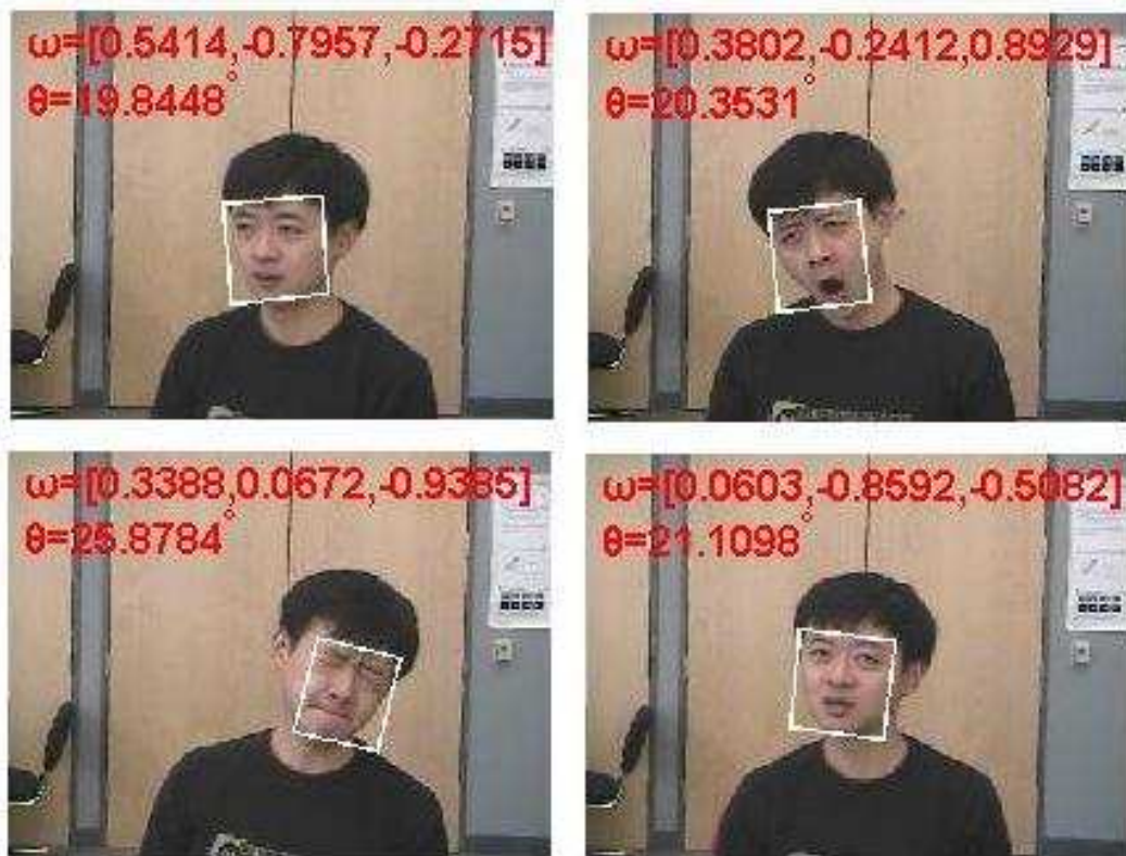
Fig. 2. An example of face tracking under changes of pose and expressions. The estimated pose is shown on the top of the frames. The pose is represented as a unit vector for the rotation axis, and the rotation angle in degrees, where the reference is taken to be the frontal face.
