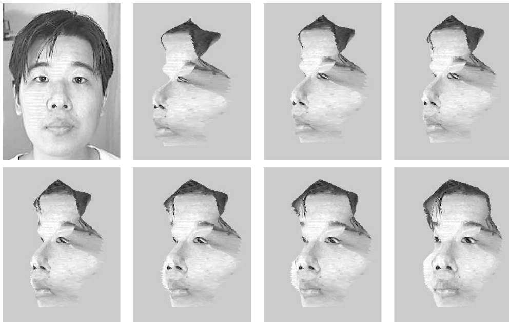
Figure 2. One frame from the original video sequence followed by the reconstructed 3D model viewed from different positions using the SIS procedure.
