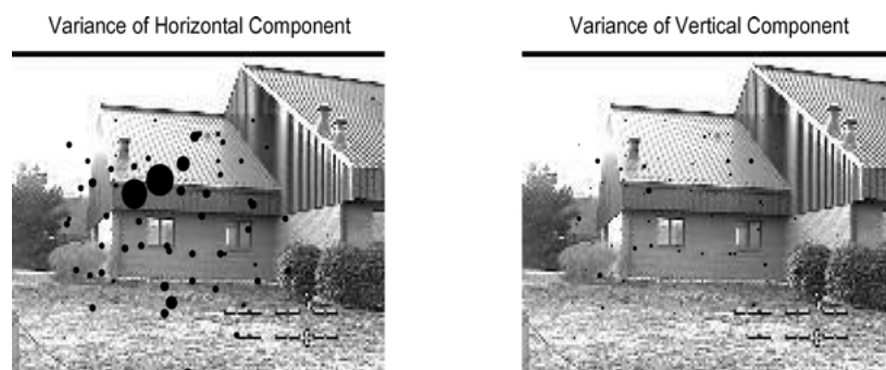
Figure 10. Plot of the variances of the feature correspondences in an outdoor sequence. The variance is represented at the corresponding feature point in the image. The diameter of the circle is proportional to the variance for that feature point. One of the plots is for the variance in the horizontal component of the motion for that feature, while the other is for the vertical component.
