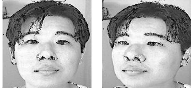
Fig. 2. Result of the corner finder algorithm on two images is represented by the small dots.
