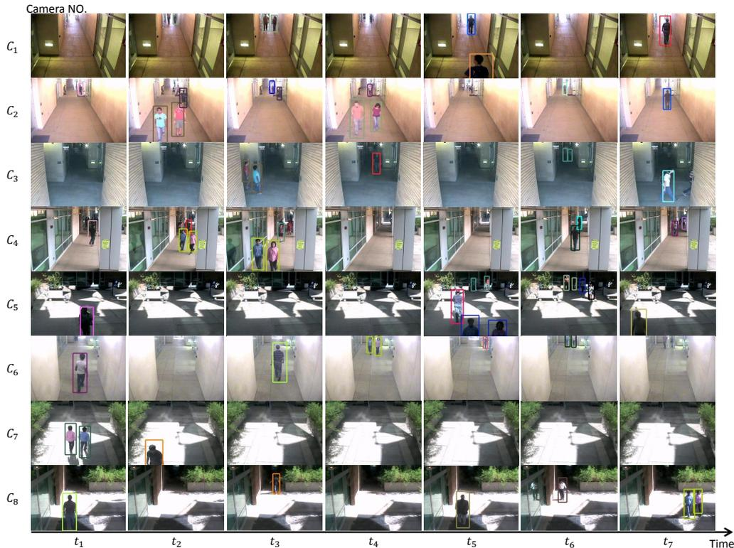
Figure 5. Tracking result of scenario 1. Each row is the view from a different camera. Each column is a snapshot from all the cameras at a particular time instant. Bounding boxes of the same color from one time instant to the next represent re-associated targets. Bounding boxes of the same color within camera views represent a collection of people recognized as a group.
