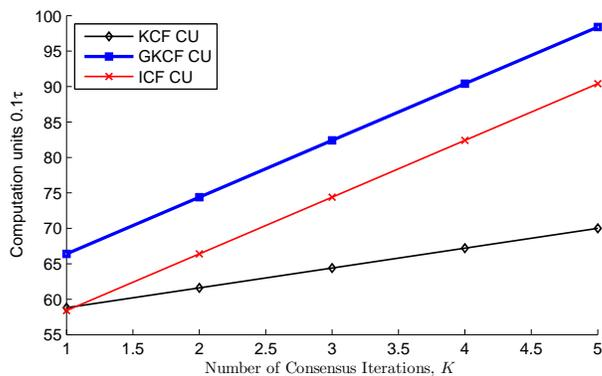
Fig. 8: Computation unit  $\tau$  vs. number of consensus iterations  $K$  for different approaches.
