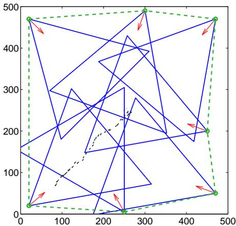
Fig. 3: In this image of an example simulation environment, the red arrows indicate the locations and orientations of the cameras. The camera FOVs are shown in blue triangles. There are 7 cameras in this example. The green dotted lines represent the network connectivity. Each black arrows depict the actual trajectory of a target moving on the grid.
