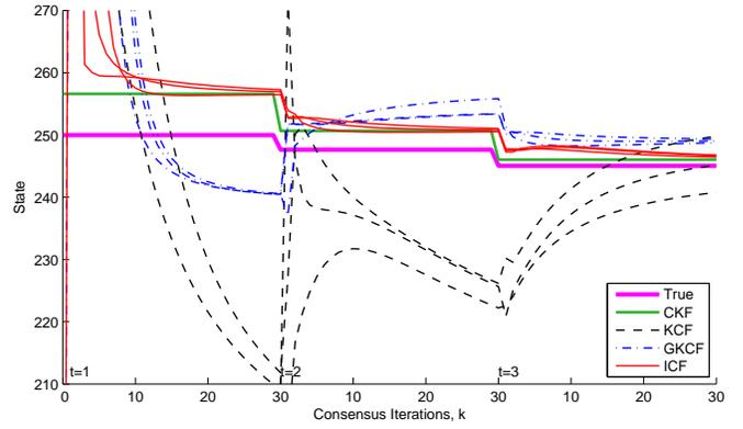
Fig. 2: An example showing the convergence of different algorithms with multiple consensus iterations at different time steps.
