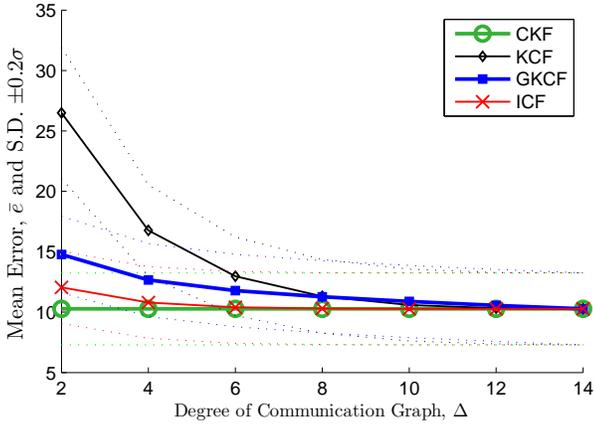
Fig. 11: Performance comparison of different approaches as a function of the degree of communication graph,  $\Delta$ . Increase in network connectivity increases the performance of all methods.
