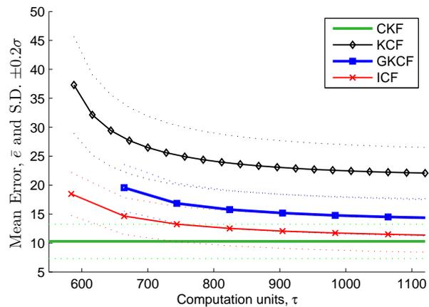
Fig. 10: Performance comparison between different approaches as a function of the computational unit  $\tau$ , showing that the ICF performs better than other distributed approaches at each  $\tau$ .
