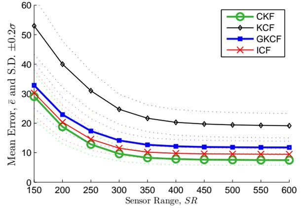
Fig. 12: Performance comparison of different approaches by varying sensor range,  $SR$ . As the sensor range increases, the network gets more measurement information and has fewer naive nodes increasing overall performance of all methods (including centralized).
