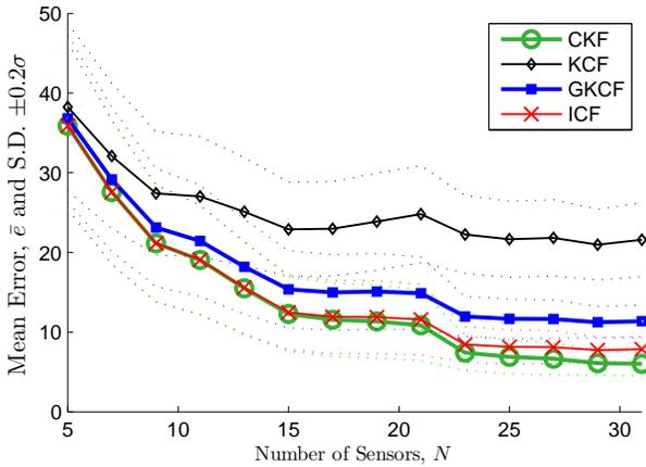
Fig. 13: Performance comparison of different approaches by varying total number of sensors,  $N$ .
