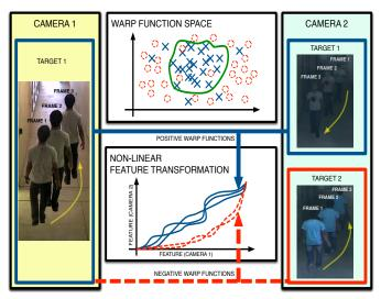
Fig. 4. Re-identification by discriminating in the warp function space. The warp functions computed between features extracted from images of the same target (i.e. positive warp functions) are shown in solid blue. The warp functions computed between features extracted from different targets (i.e. negative warp functions) are shown in dashed red. A nonlinear decision surface (shown in green) is learned to separate the two regions.
