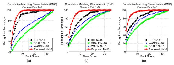
Fig. 9. CMC curves for the WARD dataset. Results and comparisons in (a), (b) and (c) are shown for the camera pairs 1-2, 1-3, and 2-3 respectively. All the results are reported for the case where the dataset is split in terms of persons with N=10.
