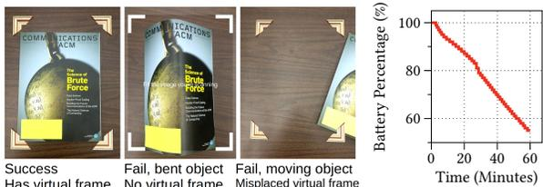
(a) ARCore [20] object detection fails for non-affine transformations. (b) Frequent DNN executions drain battery.
